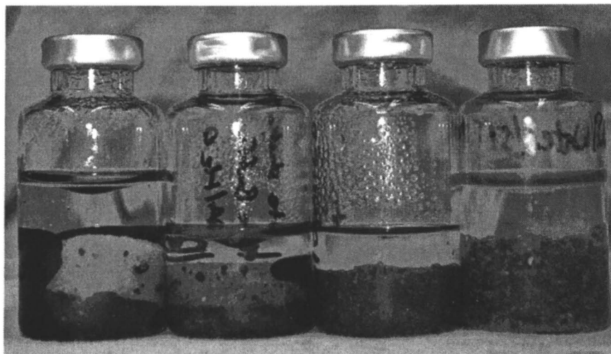
Figure 3. Bottle point experiment illustrating the effect of mineral coatings on wettability alterations. From left to right: (1) quartz + pure PCE + H 2 O, (2) hematite + DDA + PCE + H 2 O @ pH = 5.19, (3) quartz + DDA + PCE + H 2 O @ pH = 5.19, and (4) quartz treated with Rhodorsil 51T + pure PCE + H 2 O.
